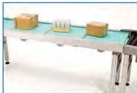
Product jams and side by side products eliminated with belt surface
